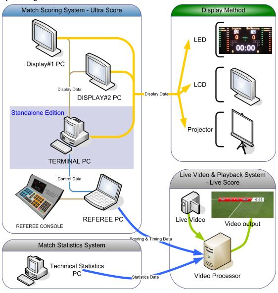
This system is composed with several modules, they are: Terminal, Remote Display.
